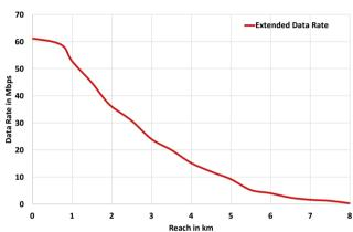
Rate/Reach Performance Measurement of Intel® SHDSL Chipset. Extended Data Rate, crosstalk-cancelled, sequential startup, 4-pair bonding, standard twisted copper pair phone cables, no alien noise
